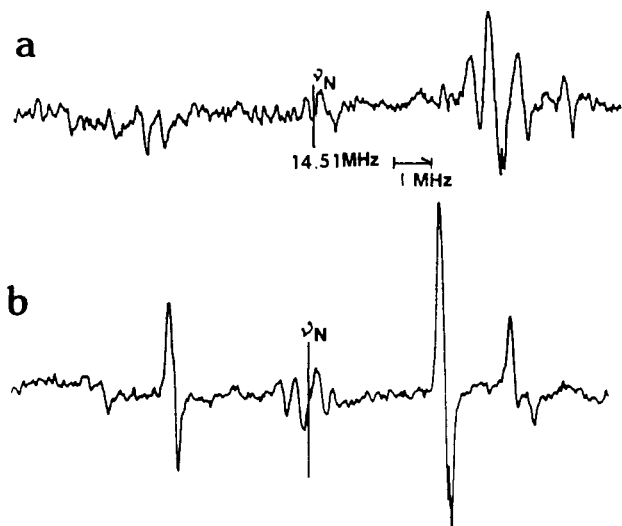
Figure 3. Proton-ENDOR spectrum of (a) \alpha -anisyl-4-methylbenzyl tert -butyl nitroxide ( 2 ) and (b) \alpha -cyclopentylbenzyl tert -butyl nitroxide ( 3 ) in water at 290 K. Spectrometer settings are the same as those in Figure 2.
